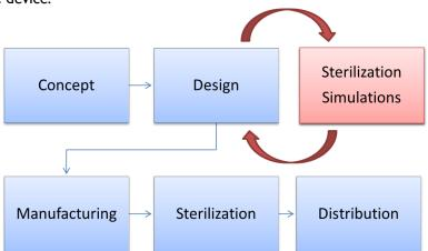
For instance, what if the material of a component in the product is changed? How is the resulting dose distribution influenced? Simulations provide direct access to this information by providing a systematic way to test such design choices. In this way, the product's ability to meet the sterilization regulations can be anticipated and actively managed.
